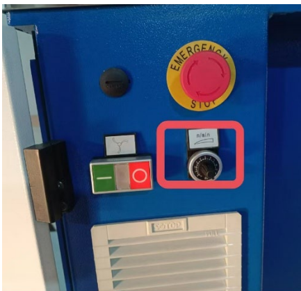
Variable speed knob to control motor speed
