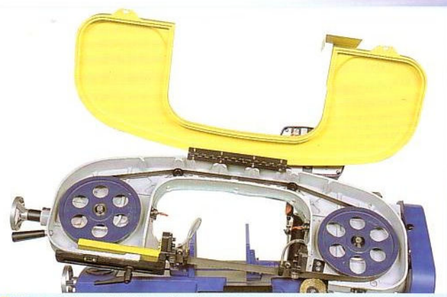
■ The plastic blowing formed blade cover decreases noise in operation.
