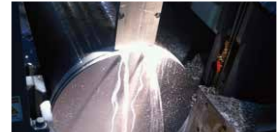
Automatic centering compact coolant supply unit is able to cool cutting area directly. (Patented)
