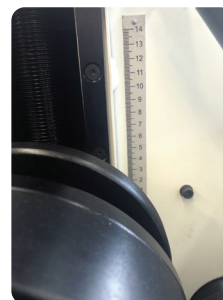
SCALE ON SIDE OF TOP ROLL FOR POSITIONING
