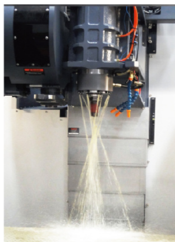
Spindle Annular Coolant Jet with 8 Nozzles
