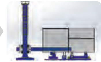
D、内环缝焊接 D、Inner circular seam welding
