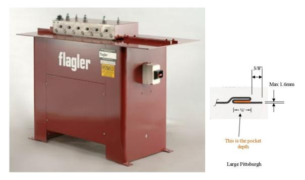
This machine is designed for heavy gauge Pittsburgh locks. Complete with hardened feed gauge, 3 piece roll/shaft/gear construction, and calibrated dial for 16-20 Ga. mild steel.
