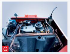
Hydraulic System Pressure adjusted via relief valve. Variable speed achieved via a rotary valve.
