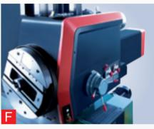
Protective Enclosure Welded high quality steel plates form an excellent protective cover.
