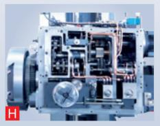
**Headstock** Primary speed is controlled via switches on the headstock itself, a variety of rotational speeds are possible.
